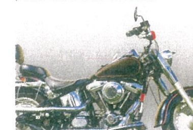
Figure 21 This Harley-Davidson motorcycle uses chrome-plating for corrosion protection and decorative effects.
