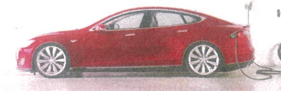
Figure 29 Tesla Model S. This All-Wheel Drive Dual Motor electric vehicle uses lithium-ion battery technology. It is capable of accelerating from zero to 100 kph in as little as 3.4 seconds and has a range of up to 502 kilometres. Image courtesy Tesla Motors, Inc. Alexis Georgeson.
